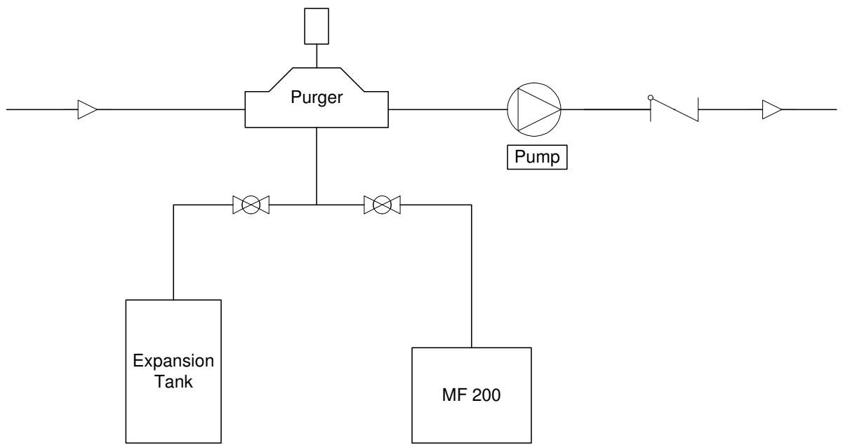
Connection Schematic – MF 200 Packaged System Feeder
